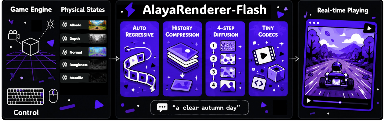
Figure 2 System overview of AlayaRenderer-Flash. During gameplay, the player independently controls game interaction through standard game inputs and visual appearance through text prompts. The game engine continuously updates the world state and exports synchronized G-buffers, which, together with the text prompt, are processed by AlayaRenderer-Flash to generate stylized RGB frames in real time. The rendered frames are immediately displayed to the player, forming a closed-loop interactive rendering system.
