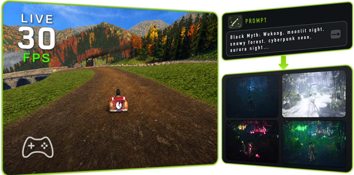
Figure 1 AlayaRenderer-Flash restyling a live SuperTuxKart session in our interactive web demo. The game engine continuously exports synchronized G-buffers to AlayaRenderer-Flash, which generates stylized RGB frames at playback rate. Players can modify the visual style of the rendered game through arbitrary text prompts while the underlying gameplay logic remains unchanged.
