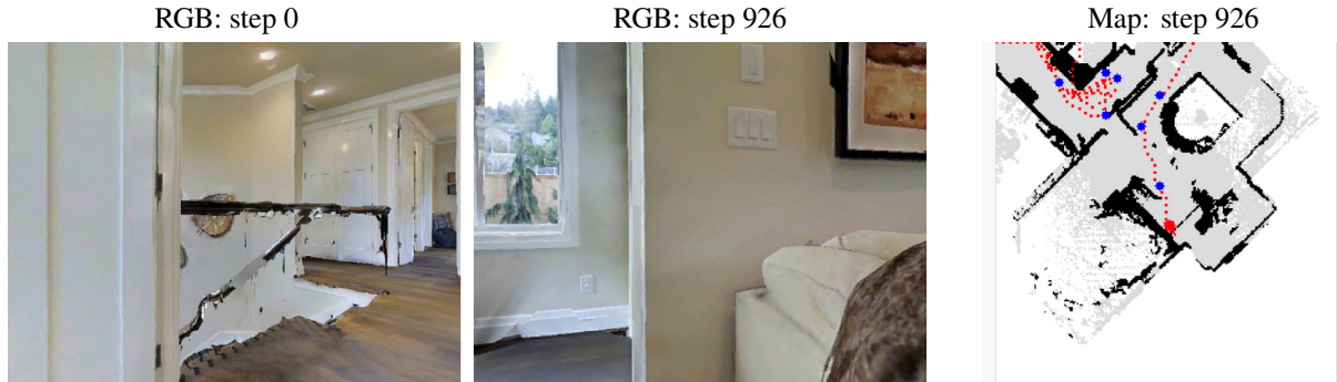
Figure 6. RxR 154: a long instruction-following rollout. The route proceeds from stairs through dining and kitchen areas to a corner near a glass door. The projected-target check passes at step 925 (0.49 m), and the episode succeeds at step 926 with a terminal goal distance of 0.43 m, within the 1,000-step budget.
