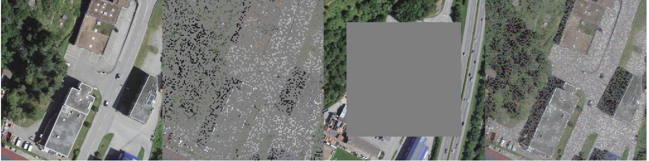
Figure 2. Self-supervised inference results on the CASWiT architecture. Each image (left to right) shows: original high-resolution image, high-resolution image with random masking, low-resolution image with central masking, and the reconstruction of the high-resolution image after SimMIM-style pretraining.
